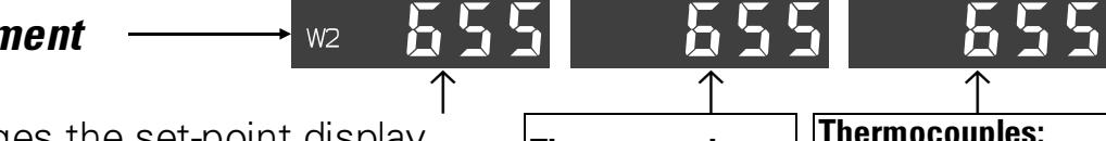
Pressing keys **▲▼** changes the set-point display (the longer the faster). The modification is effective after 2 s or by pressing **□**.
