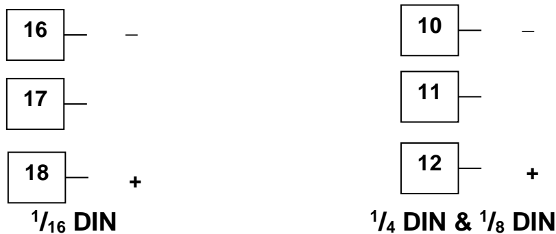
Figure 31. Option Slot 3 - Transmitter Power Supply Module
